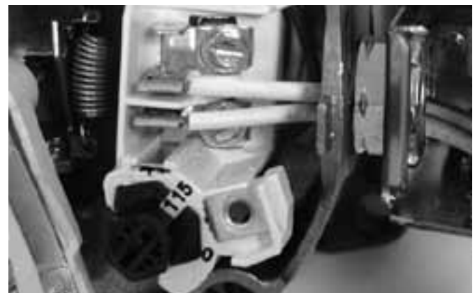
Figure 11: Voltage set to 115 volts, Dial Type
